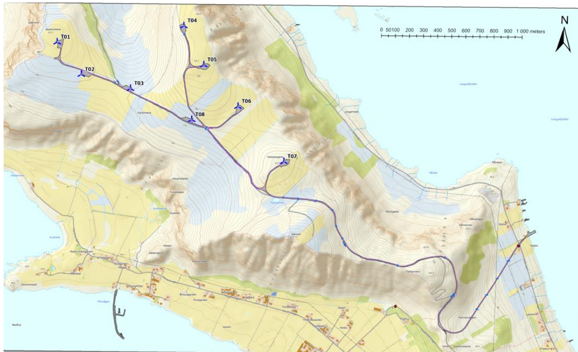
Figure 1. Location and numbering of Haramsoya wind turbines. Measurements was carried out for the wind turbine T07.
