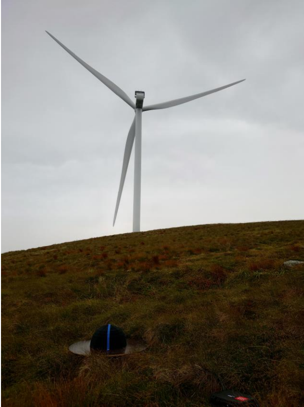
Figure 1-2: Wind turbine T07 and sound level meter with measurement board and secondary windscreen.
